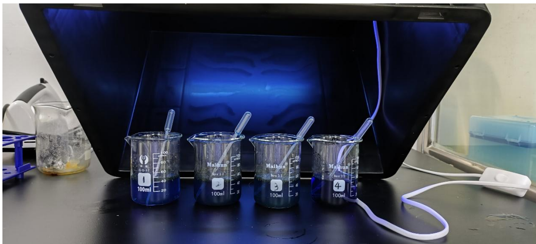
Figure 3 Photocatalytic adsorption-degradation experiment for methylene blue
