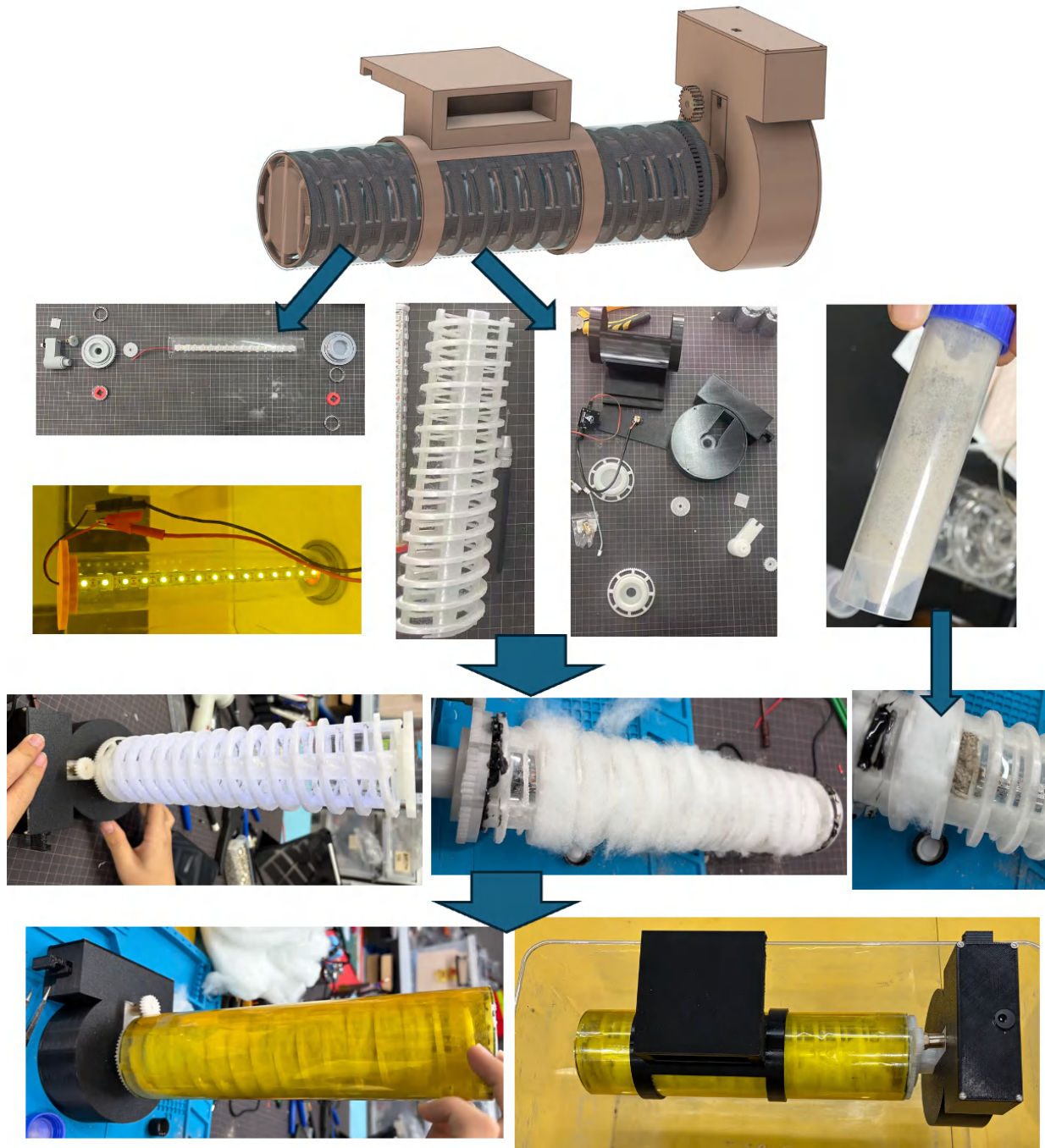
Figure 5 Archimedean screw reactor prototype building process
